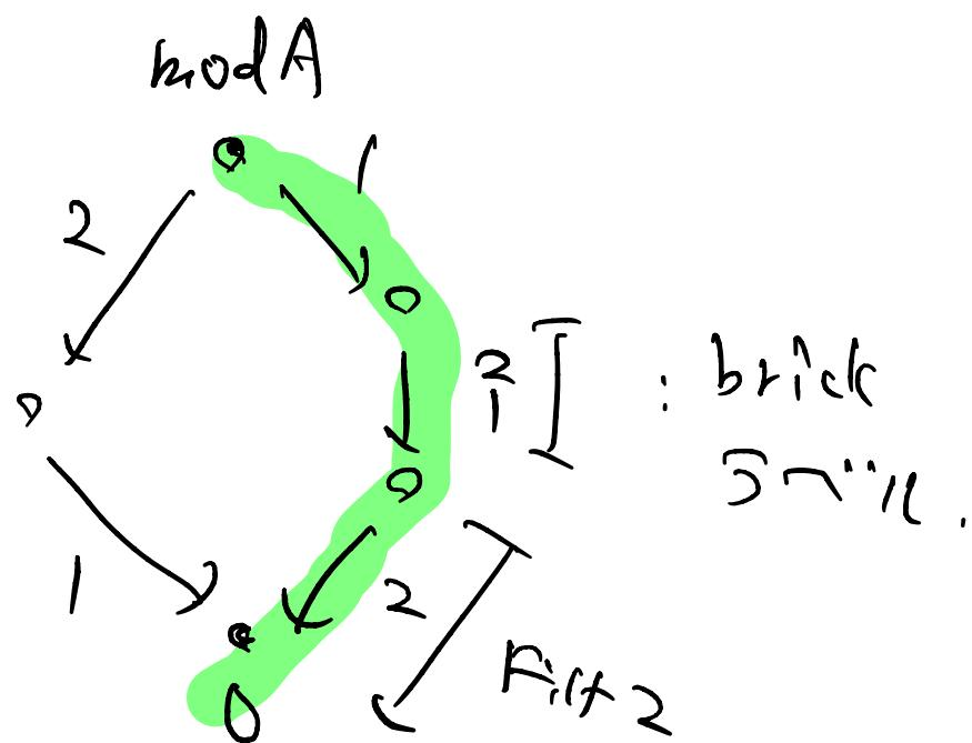
$$\text{mod } A = F_{\text{filt}} 2 * F_{\text{IH}}^2 * F_{\text{HT}} 1.$$
